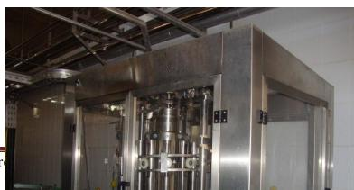
Tunnel for cooling and pasteurizing the cans after filling provided with 7 pumps feeding the tunnel from the pasteurizer + 2 pumps for the tunnel + electrical panel 304S.S all included.
