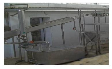
3. A collection of conveyors for cans before and after filling and closing 304S.S provided with complete PLC connectors and its accessories.
