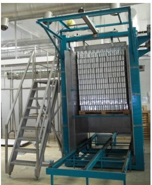
2. Conveyor for feeding the empty packets 304S.S provided with packets washing machine and water pump 2KW power and automatic steam valves and hand
