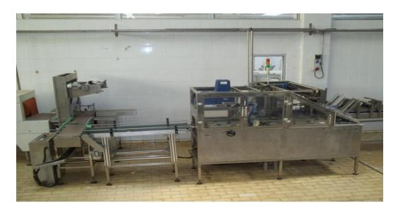
• Labeling machine provided with motor 1.5kw power.
