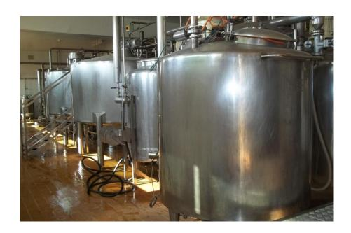
2 tanks (316S.S) for preparing the juice 3000L capacity, each tank provided with mixer with gearbox 3hp and pneumatic valve 2 inch out of tank + Ladder S.S + Level Sensor.
