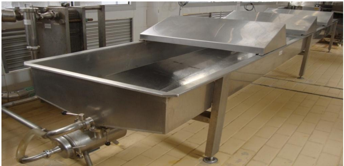
4. Drum sifter provided by pulling pump + Electrical panel + Motor 0.75 KW + Pump 4 KW.
